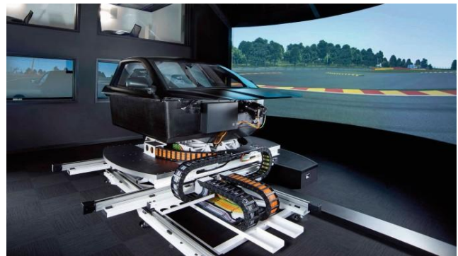
Fig. 3. Driver-in-the-loop (DIL) simulation for autonomous vehicle testing [41]
