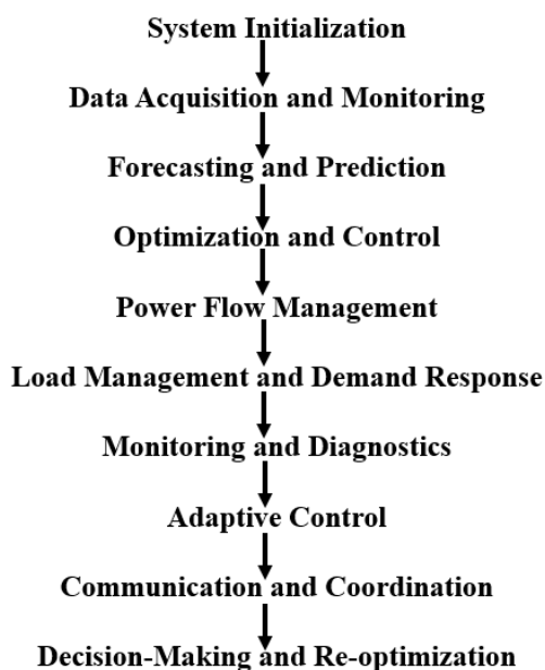
Fig. 1. Process diagram of an algorithm for hybrid energy generation
