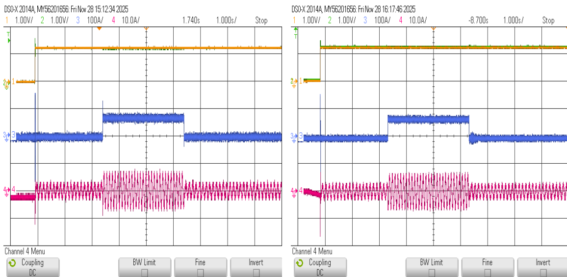
Fig. 11. Real-time constant speed responses under load disturbance for RBFPI SM (left) and RBFPI STASMRC (right): speed, electromagnetic torque, and phase-a current
