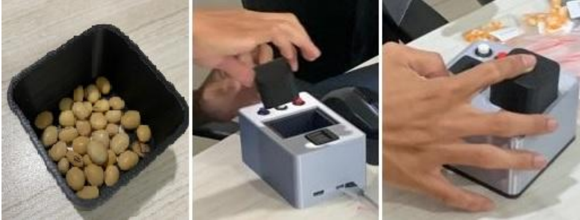
Fig. 6. Vis/NIR spectral data acquisition process for soybean seeds
