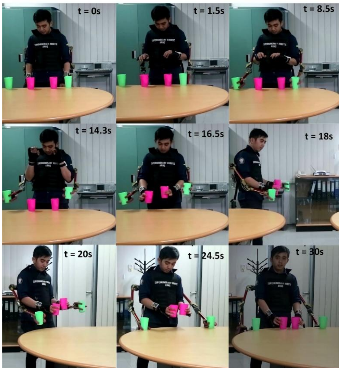
Fig. 10. Cooperative object manipulation task between biological arms and extra arms
