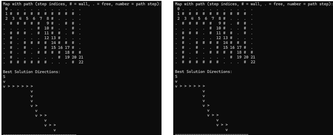
Fig. 17. Best paths obtained by A* and backtracking for map11
