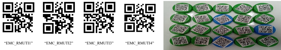
Fig. 4. Definition and assignment of unique QR code identifiers for workpieces
