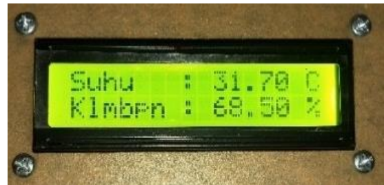
Fig. 7. LCD display, suhu (Temperature), Klmhpn (Humidity)
