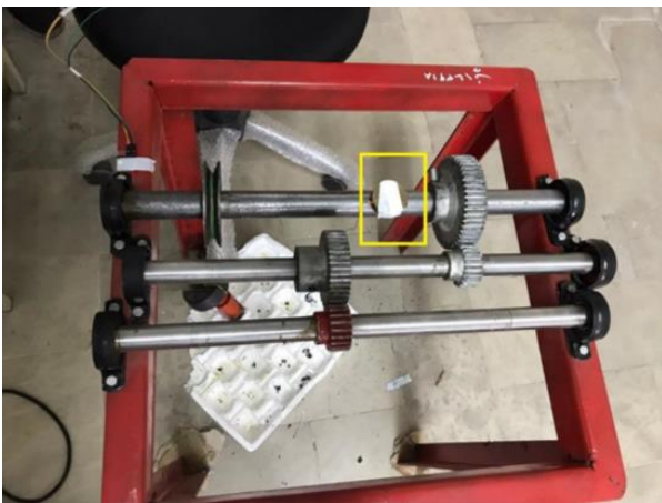
Fig. 11. Unbalance mass appended at the shaft
