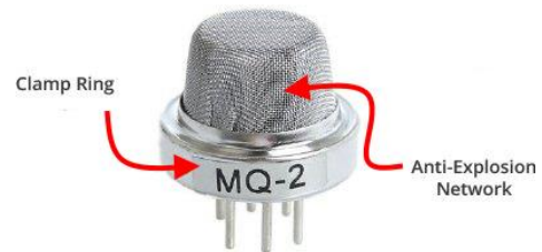
Fig. 3. Structure of MQ-02 gas sensor
