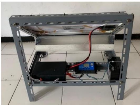
Fig. 5. Solar panel framework from rear view
